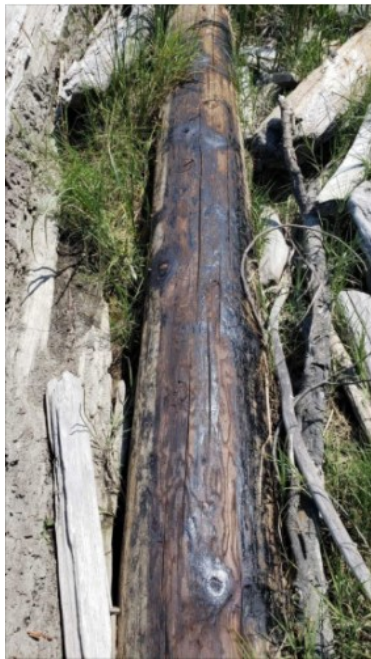
A large creosote log found in Livingston Bay, Port Susan. Notice the shiny, tar-like creosote on the surface of the log.
