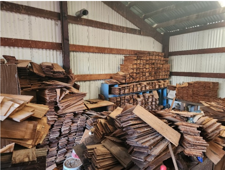
Photo 40: Inside the finishing building, piles of finished product can be seen. The pipe in the photo connects to the next room, used to transport vacuumed sawdust.
