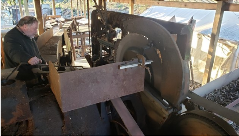
Photo 14: The saw used to cut cedar shake and shingles—A 1916 saw manufactured by Sumner Iron Works in Everett, Washington. The conveyor belt carrying sawdust away can be seen in the bottom right of the photo. The sawdust was carried to an incinerator just to the north of the mill.
