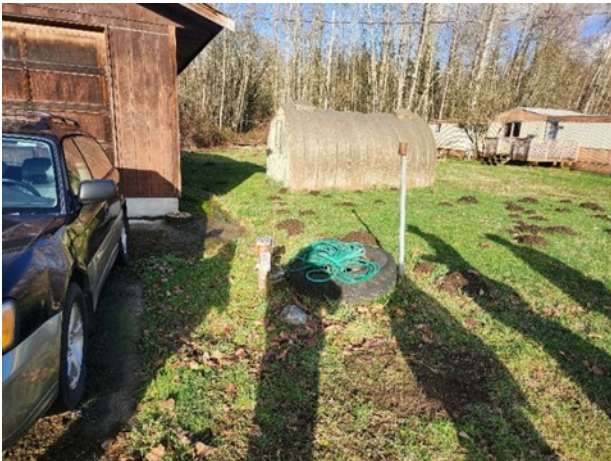
Photos 23 & 24: Next to the garage, there is an Underground Storage Tank containing gasoline. Owner claims the tank was likely pumped out by his father following the closure of the mill. However, the vent pipe smelled like product was still present. The tank is presumed to be 4-5' long and 3' wide.
