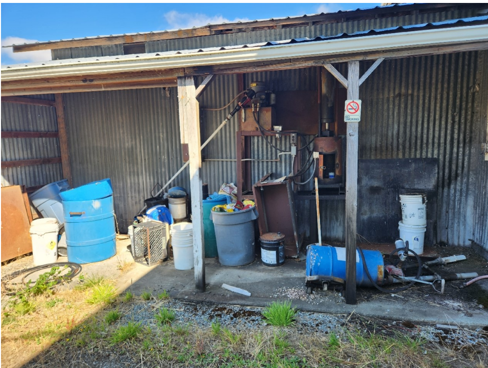
Photo 8: An oil filter recycling area. Twin City Foods staff utilized a hydraulic press to crush used oil filters and squeeze out any remaining oil. There were surface-level oil stains seen around the station. Steve Karcher (employee of TCF) said this recycling station hadn't been used in years, so a catch basin may have been used when in operation, but couldn't be determined during our survey. The oil/fluid storage room in the main shop is located on the other side of the wall pictured. Photo was taken looking north. Map Photo ID: 48
