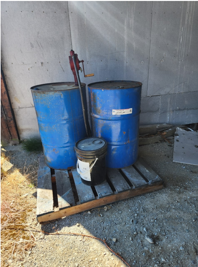
Photo 27: Within one of the pole barns, staff identified two 55-gallon drums which contained unleaded gasoline and/or red dye diesel. Staff did not identify oiled soils around this area. Map Photo ID: 78
