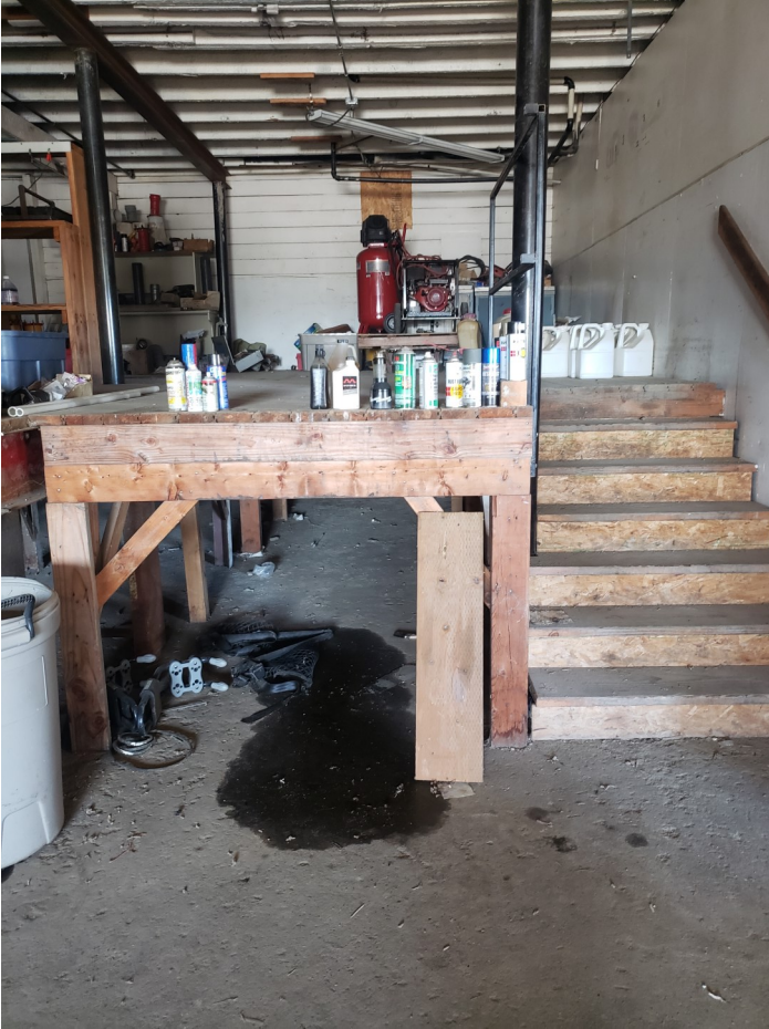
Photo 35: An oil stain, bottles of unknown fluids, aerosol cans, and an air compressor found in the second shop.
